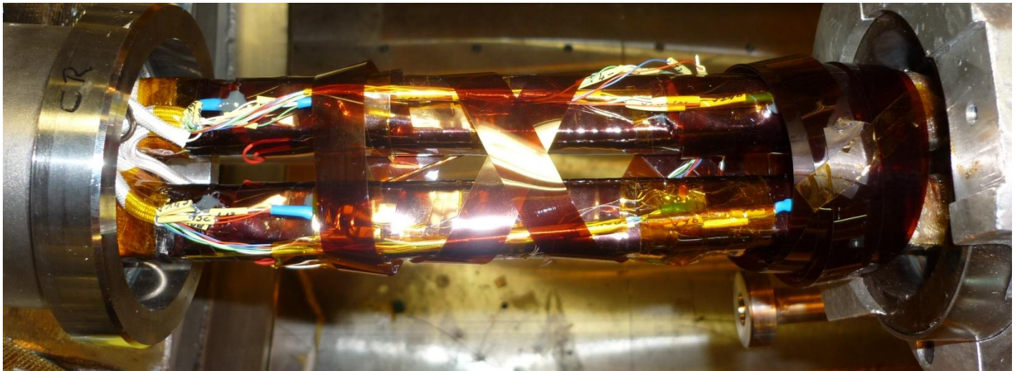
Figure 39. The M3 interconnection after preparing the insulation and instrumentation.
