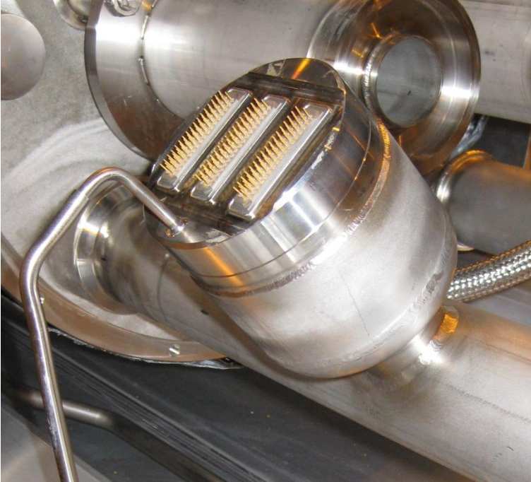
Figure 50. Connection box close-up with the all-important tube (left-bottom) to pump the chamber inside the box vacuum.
